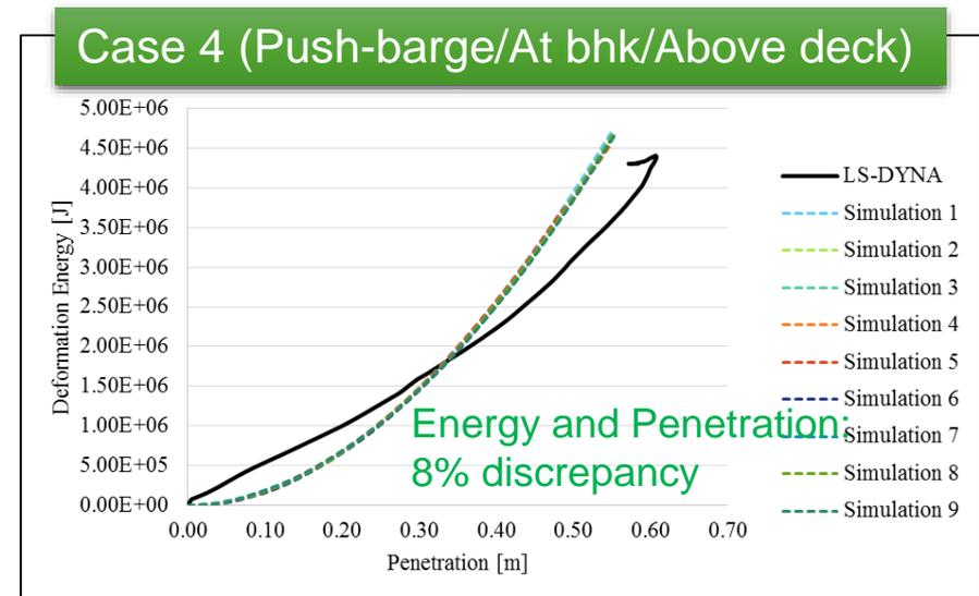
➤ **Some of the results with rupture strain (A.D.N. Regulations)\*\*\***
